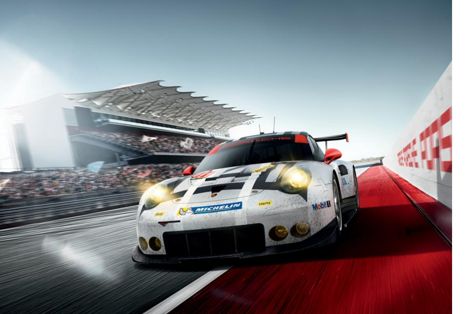
From the very start, the 911 RSR was designed with long-distance racing in mind. Honed over more than 50 years, the unmistakeable 911 silhouette reflects the pure power that is just waiting to be unleashed. The water-cooled six-cylinder Boxer engine with four-valve technology transmits its power output to the rear axle via a specially developed six-speed sequential Porsche GT racing gearbox.
